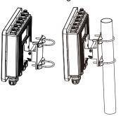
Step 5 Adjust device position and tighten the derrick nut to fix the position of the device on the derrick. Installation ends.
