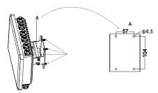
Step 5 Install the device on the wall and tighten the screw. Installation ends.
