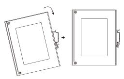
Step 1 Check whether the DIN-Rail mounting kit that comes with the device is installed firmly.
