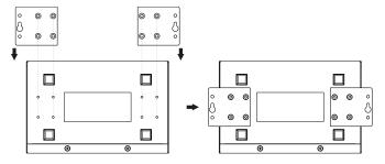
Step 2 On the wall of device mounting, place the device on the wall for reference or refer to the mounting dimension to mark two screw positions.
